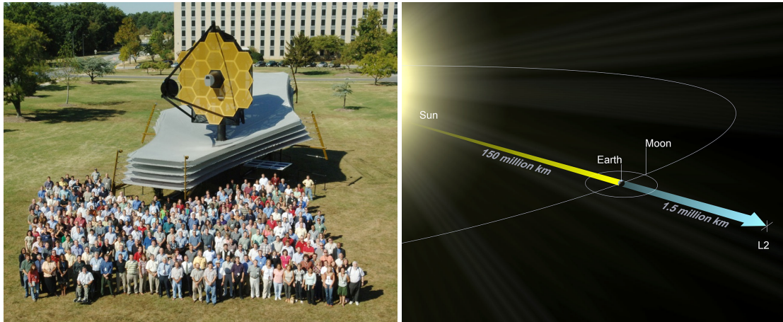
Figure 5: Left: A full-scale model of JWST next to some of the scientists and engineers involved in its development at the Goddard Space Flight Center. Credit: NASA / Goddard Space Flight Center / Pat Izzo. Right: The position of the second Lagrangian point, L_2 , relative to the Earth. Credit: ESA.
